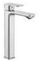
MABM103 Single Lever Basin Mixer with Extended Body without Pop-Up Waste System (Length of Spout: 6.1 inches Height of Aerator: 9.3 inches)
